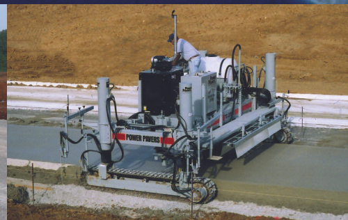
Power Paver TC 2700 Adds texture and cures concrete
