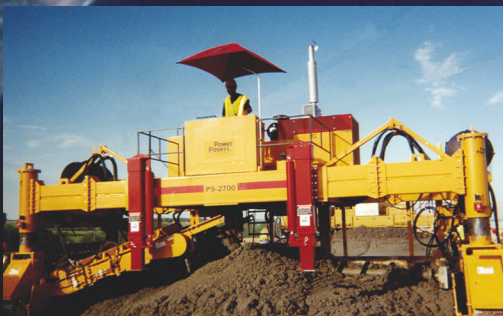
Power Paver PS 2700 Places and spreads concrete
