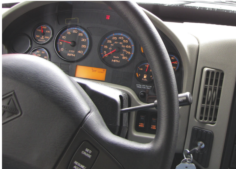
Water-temp gauge (left of the tach) on the WorkStar stayed at 180 degrees and edged just above that at the end of a suburban run, showing the MaxxForce DT was running cool.
