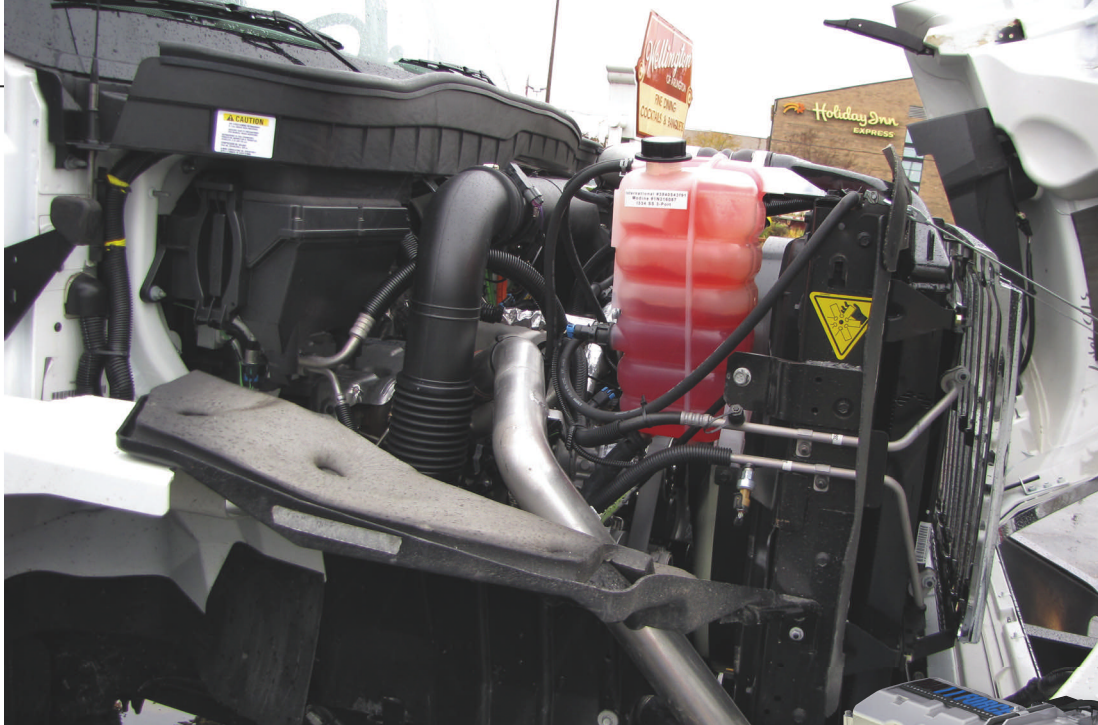
Under the hood, the midrange MaxxForce DT is hidden behind turbos, pipes, filters and a fluid bottle. Cooling module includes two-core radiator.
