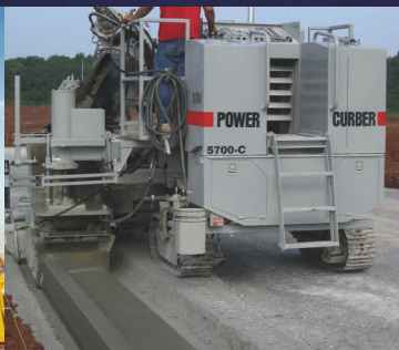
Power Curber 5700-C Curb and gutter, sidewalks
