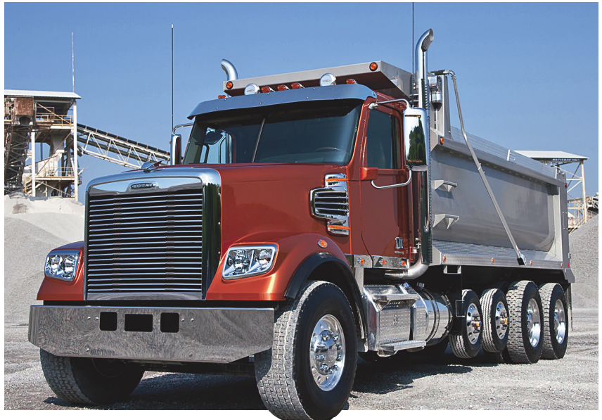
Coronado SD can be ordered as a tractor or straight truck. It will use EPA-'10 diesels from Detroit and Cummins with exhaust systems that allow for easy mounting of dump beds and other bodies.
